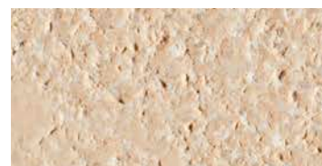
bocciardato / bush-hammered / gestockt
