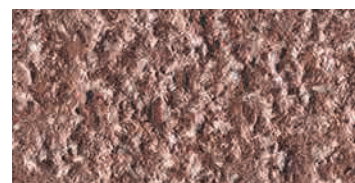
bocciardato / bush-hammered / gestockt
