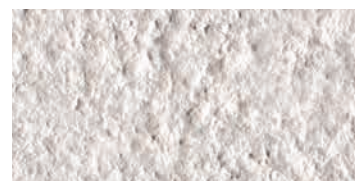
bocciardato / bush-hammered / gestockt
