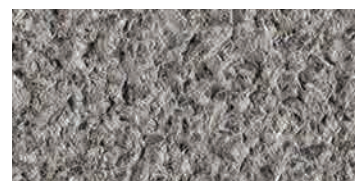
bocciardato / bush-hammered / gestockt
